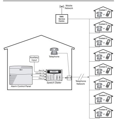
The Speech Dialler provides a means of communicating alarm information from an alarm control panel to a standard or mobile telephone. The unit is normally connected to an alarm control panel, which provides the necessary power and battery backup. The unit is also connected to a standard telephone line and behaves like another extension to the telephone and does not affect its normal operation or that of any other extension fitted.
